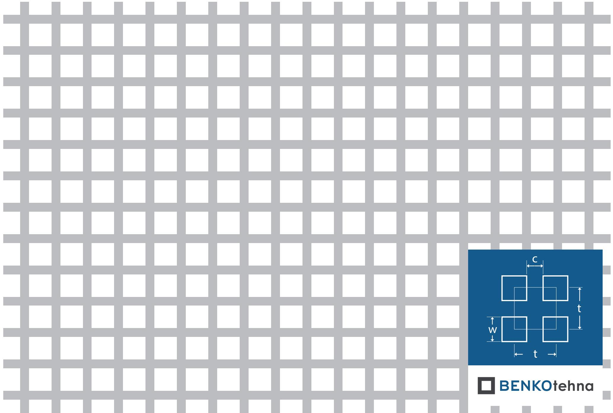
Kvadratna vrstna Kv 10-14:  $w = 10,0 \text{ mm}$  |  $c = 4,0 \text{ mm}$  |  $t = 14,0 \text{ mm}$  | odprtost = 51,02%
