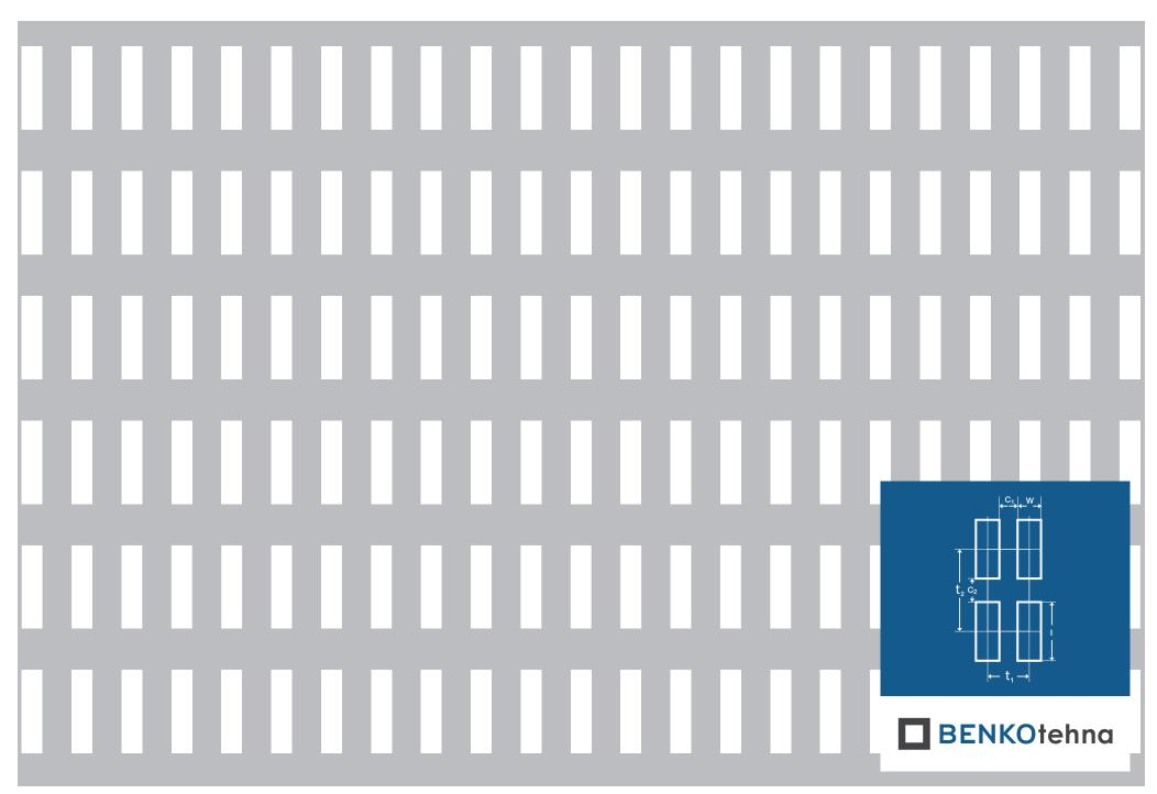
**Podolgovata vrstna Pv 5×20-12×30:**  $\mathbf{w} = 5.0 \text{ mm} \mid \mathbf{c_1} = 7.0 \text{ mm} \mid \mathbf{c_2} = 10.0 \text{ mm} \mid \mathbf{t_1} = 12.0 \text{ mm} \mid \mathbf{t_2} = 30.0 \text{ mm} \mid \mathbf{l} = 20.0 \text{ mm} \mid \mathbf{odprtost} = 27.78\%$
