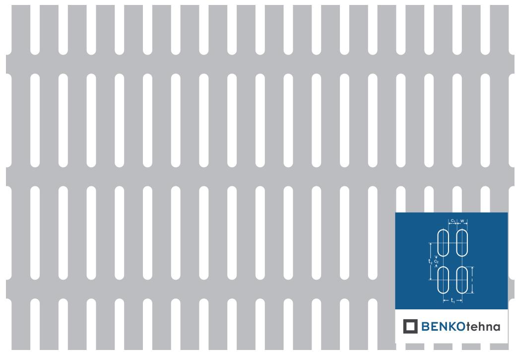
**Podolgovata vrstna Pv 5×50-15×60:**  $\mathbf{w} = 5.0 \text{ mm} \mid \mathbf{c_1} = 10.0 \text{ mm} \mid \mathbf{c_2} = 10.0 \text{ mm} \mid \mathbf{t_1} = 15.0 \text{ mm} \mid \mathbf{t_2} = 60.0 \text{ mm} \mid \mathbf{l} = 50.0 \text{ mm} \mid \mathbf{odprtost} = 27.18\%$
